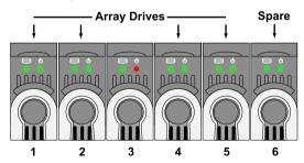
When the Manual Transition is finished, physical drives 1, 2, 4, and 5 belong to the disk array and physical drive 6 is a revertible spare drive.
